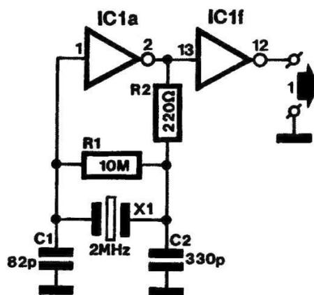
Figure 1: Oscillator circuit.
