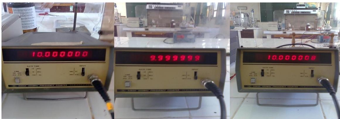
Figure 2: Displayed frequencies of 10MHz quartz oscillator
