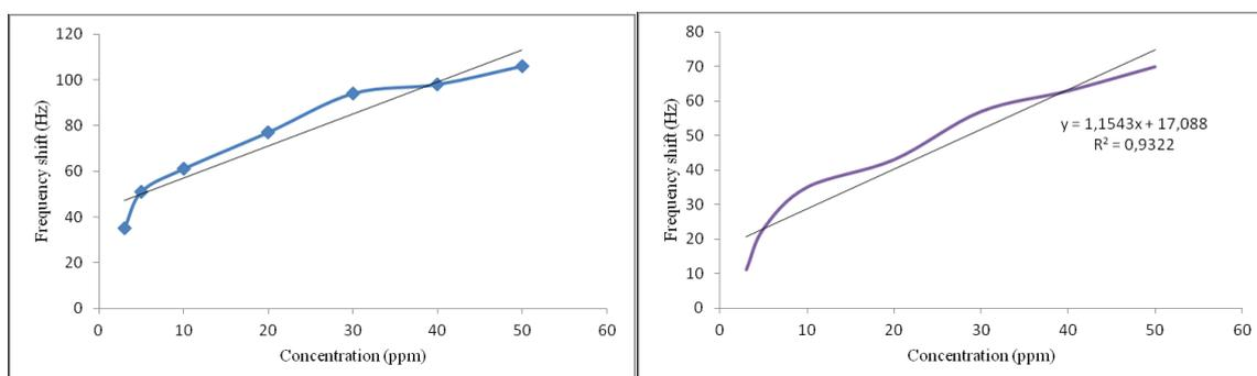
Figure 4: Linearity response in range of 3 – 50ppm (a) Water; (b) benzene
